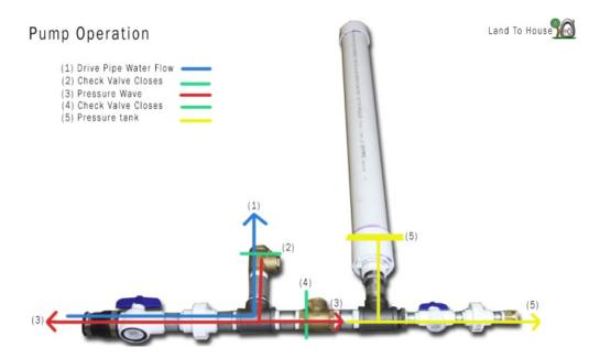
The pressure wave that is needed to get the system working correctly will not work well if the drive pipe is less than 15 feet. The pressure wave is sent back up the pipe and then out the end, thus the system does not work well or at all. This means that the drive pipe must be longer than 15 feet.
