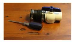
2. Gather the white pipe tape (teflon tape) and all the pipe nipples. That should be six 1-1/4" and three 3/4" pipe nipples. Place at least four winds of the white tape on the threads of each nipple. This will allow connections to be secure and water tight.
