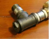
18. Connect a 3/4" pipe nipple into the bushing.
