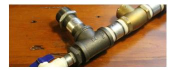
25. Screw the pressure tank to the 1-1/4" 1-1/2" bushing.
