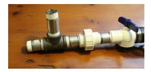
8. Up from the top of the tee, screw a 1-1/4" check valve. The direction of the water flow will need to be facing down on the check valve. There is often an arrow on the check valve that will indicate the flow direction. This arrow needs to face down. As long as the whole system is facing upright, it does not mater what angle the check valve is facing as you tighten the threads.
