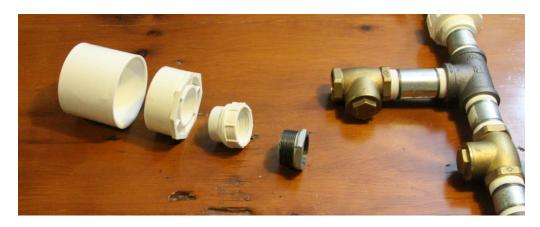
14. Use the pipe primer to coat all connections of PVC pipe. Including both ends of the 3" pipe, end cap, coupling, 1-1/2" to 3" bushing, and 1-1/2" glue bushing. These pipe sections will be glued together.
