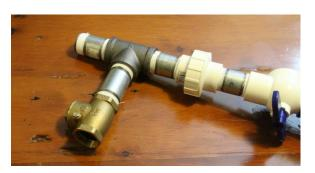
9. Place the second check valve on the other end of the tee. The direction of the water flow needs to be going out of the system. Make sure that the arrow points away from the first valve. Because gravity pulls the valve flap down it is important that the angle of the valve be upright so that the valve can remain closed naturally. What does this mean? The hinge that the valve swings on needs to be at the top of the component.
