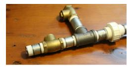
11. The next component is another 1-1/4" threaded tee. Make sure that this tee has the 90 degree angle facing upward.
