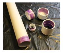
15. Use PVC cement to glue together the 3" pipe to the coupling. Then glue together the coupling to the 1-1/2" to 3" bushing. Now glue the 1-1/2" threaded to 1-1/2" glue end into the 1-1/2" to 3" bushing. Then glue the end cap to the 3" PVC pipe on the other end.
