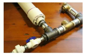
26. The basic parts of the pump are now assembled. If you are going to use a flex tube then you will need to use a rubber connector that will connect to the end of the union. If you are using a garden hose then use the connector in step 23.
