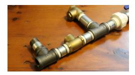
13a. If you are able to find a 1-1/4" to 3" bushing then screw the 1-1/4" to 3" bushing onto the 1-1/4" pipe nipple. Make sure that this is tight and secure because this will be the base of the pressure tank. If you are unable to find this part, see 13b.
