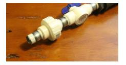
23. If you are using a garden hose as the delivery pipe, you will need a garden hose thread connector placed on the end of the last 3/4" pipe nipple.
